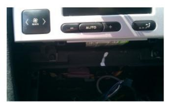
When removed the unit can be pulled out, unclip the connector and remove it fully,
