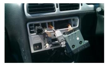
Once done, unclip the connectors from the buttons and the mfd and push the wiring back down the holes to aide removal of the surround......
